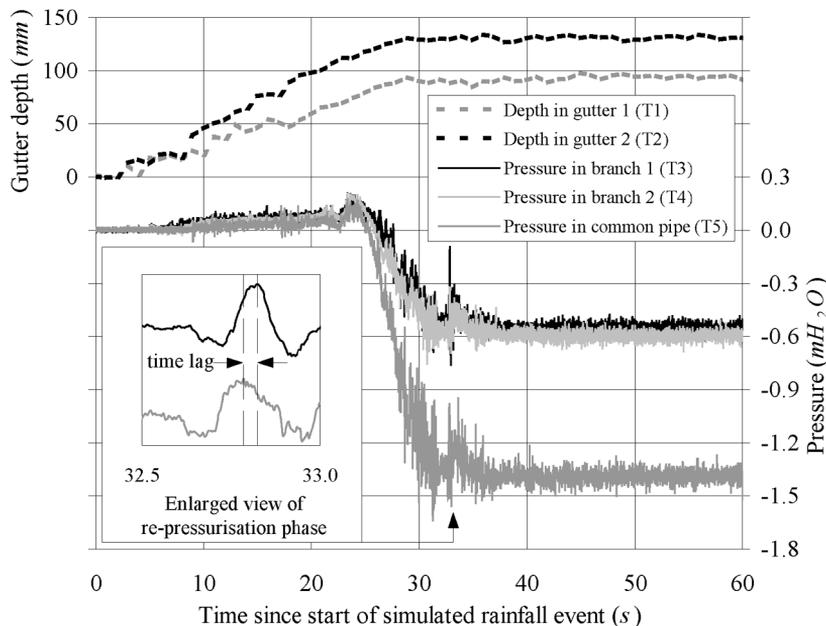
**Figure 4** Measured gutter depths and system pressures for the design criteria rainfall event (gutter 1) inflow = 5.85 l/s, gutter 2 inflow = 7.78 l/s. These data illustrates that even when fully primed (40–60 s) the pressures are not truly 'steady'.
