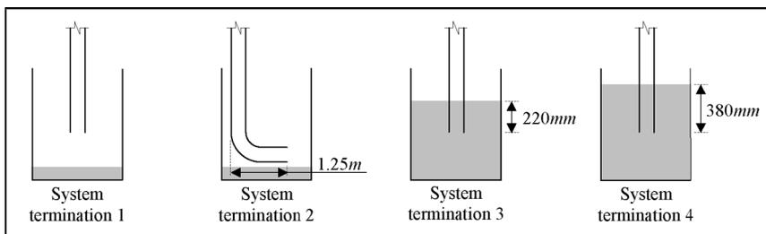
Figure 7 Siphonic system termination configurations investigated
