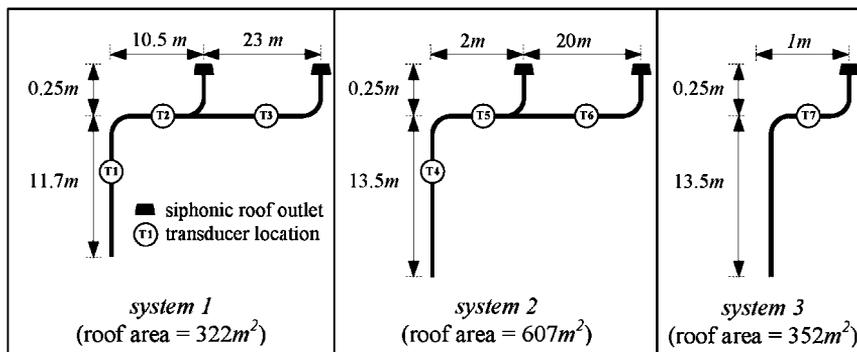
**Figure 9** Schematic of the siphonic roof drainage systems being monitored at the National Archives of Scotland Document Repository Building, Edinburgh.
