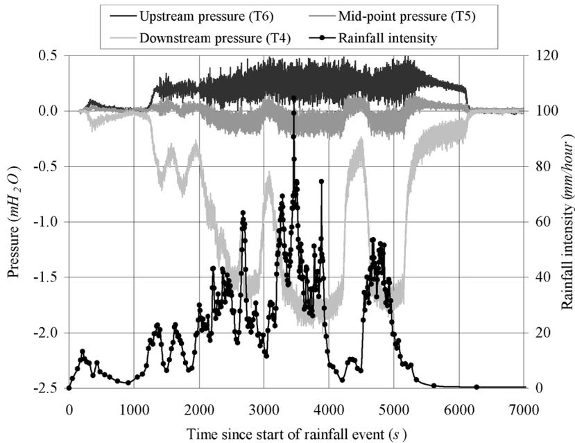
**Figure 10** Measured conditions (system 2) on 2 August 2000 (refer to Figure 9 for system and transducer layout). The time-varying nature of this rainfall event is typical, and demonstrates the importance of using rainfall hyetographs to assess system performance fully.
