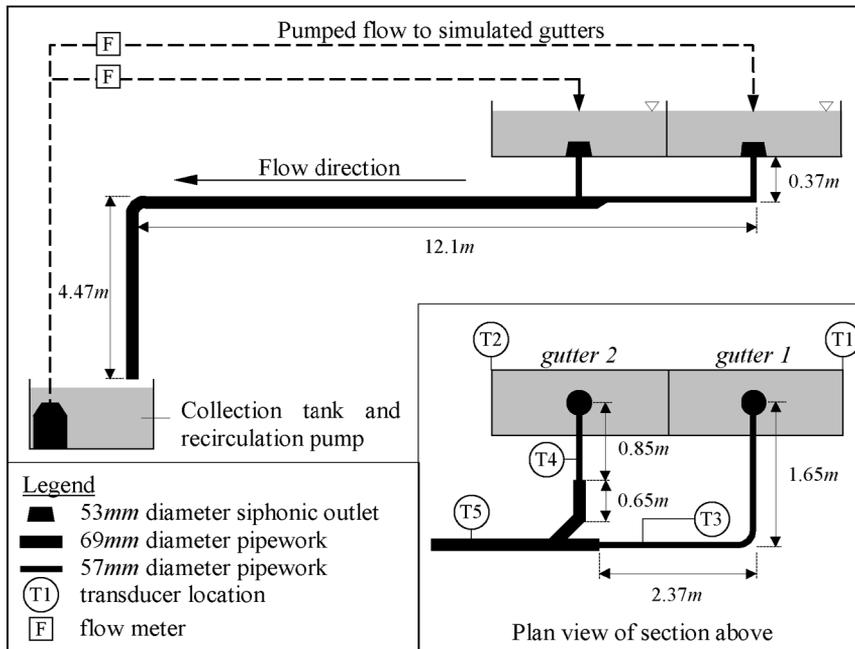
**Figure 2** Schematic view of the siphonic roof drainage test rig. The capacity of the system is the same as 75 mm/h falling on a 665 m<sup>2</sup> roof – all drained via a 69-mm diameter pipe.
