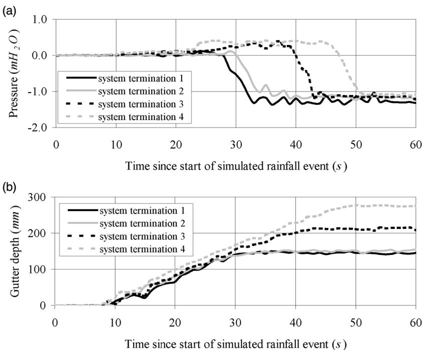
Figure 8 (a) Variation in common pipe pressure (T5) with system termination configuration (fully primed conditions). (b) Variation in gutter 1 flow depth (T1) with system termination configuration (fully primed conditions)
