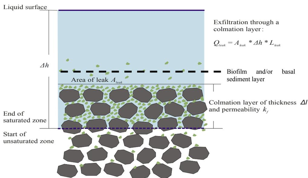
**Figure 3.** Representation of the structure and growth of the colmation layer
