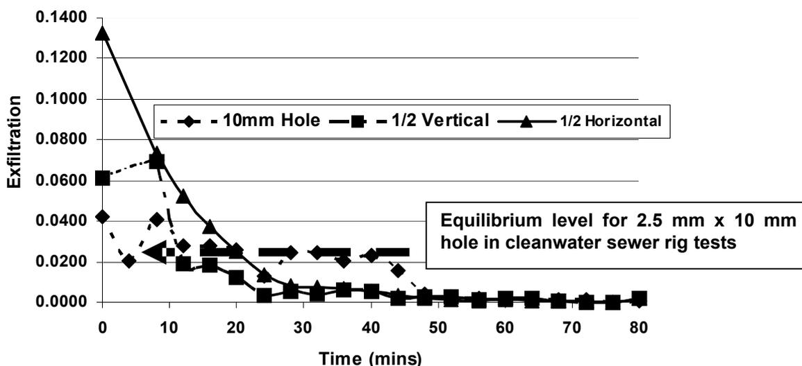
**Figure 1.** Temporal trends in exfiltration rates for varying 3 mm gap geometries and constant head (42 – 44 mm) in a live wastewater test rig. (After Blackwood *et al.*, 2005b)
