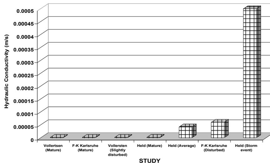
**Figure 4.** Results reported for exfiltration permeability measurements.
