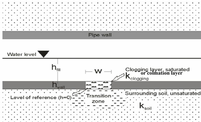
**Figure 2.** Schematic representation of a blocked leak.
